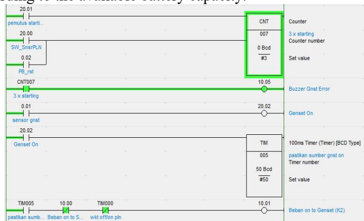
Picture 8. Cutaway ladder diagram of generator set fail on
