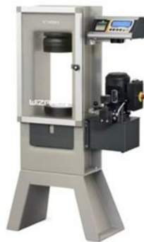
Figure 2 Concrete Compressive Strength Testing Machine
