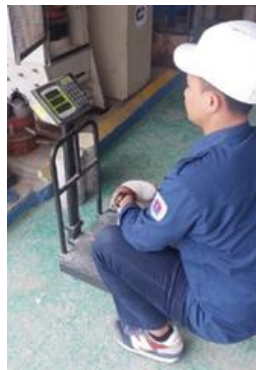
Figure 2. Process of Weighing Concrete Test Specimens
