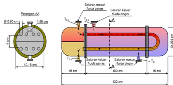
Figure 1. Dimensions and Measurement Locations
